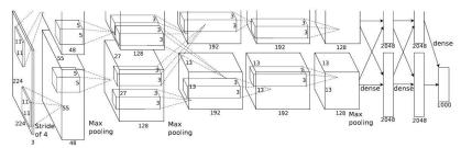
Fig. 7.10 – Network architecture AlexNet
