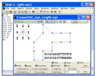
Figure 0.7. G-file for the variant of the task (Figure 0.6b) At the initial stage a number of simplifications are introduced:
