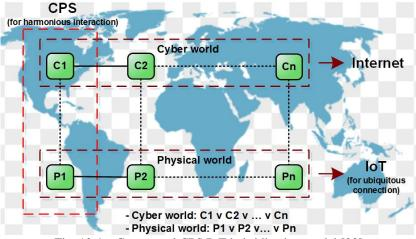
Fig. 12.4 – Conceptual CPS/IoT hybridization model [23]
