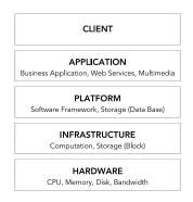
Figure 10.1 – Cloud Computing Architecture
