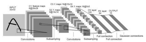
Fig. 7.9 – Architecture of convolutional neural network LeNet
