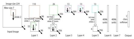
Fig. 7.12 – ZF Net Network architecture
