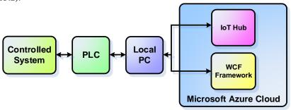
Fig. 13.1 – Proposed Architecture for Cloud Management in IoT [9]
