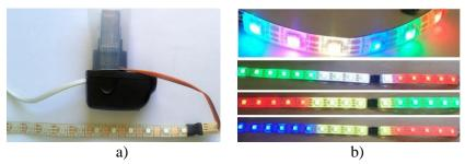
Figure 0.10. LED ribbon control module (a) and colouring options (b)
