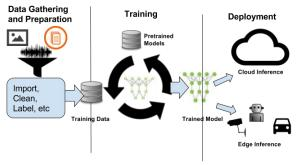
Fig. 7.19 – Basic deep learning workflow for embedded systems
