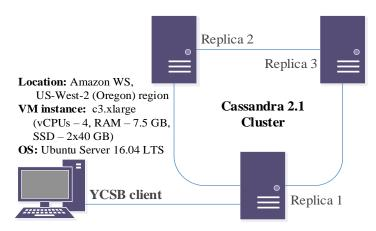
Fig. 8.3 – Experimental setup: Cassandra cluster
