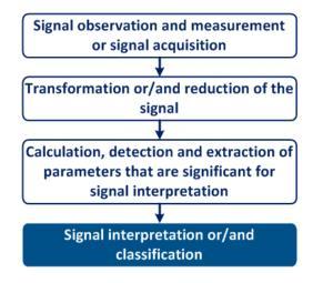
Fig. 5.6 – Processing of sensor / devices signals
