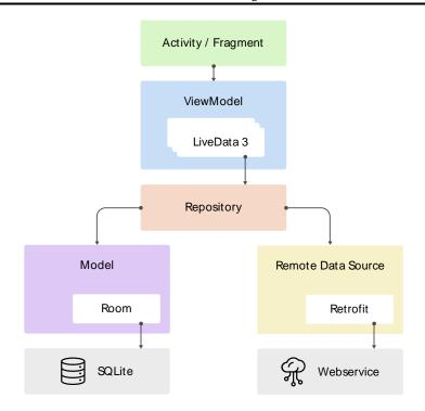
Figure 9.3 – Recommended Android app architecture
