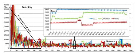
Fig. 8.5 – A fragment of the WRITE delay graph, 500 threads
