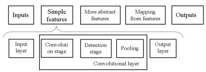
Fig. 7.20 – DNN architecture for pattern recognition
