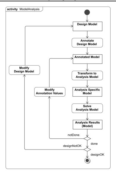
Fig. 15.11 – The general model analysis process based on MARTE.
