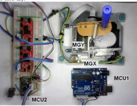
Figure 0.9. Type of mini-plotter (Homemade DIY CNC)
