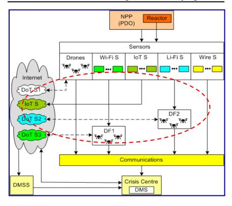
Fig.1.2. Internet of Drones based system for monitoring of severe NPP accident
