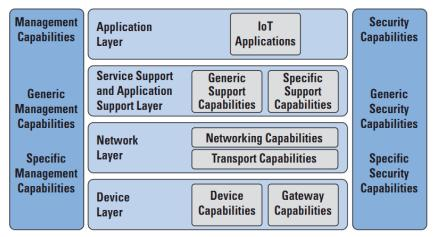
Fig. 4.1 – ITU-T Recommendation Y.2060 IoT Reference Model [1]
