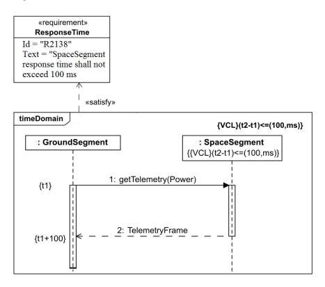
Fig. 15.10 – Example of combined use of SysML and MARTE to define requirements
