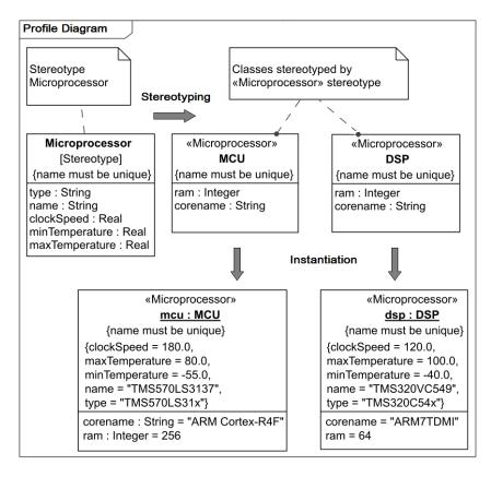
Fig. 15.1 – Example of stereotyping process
