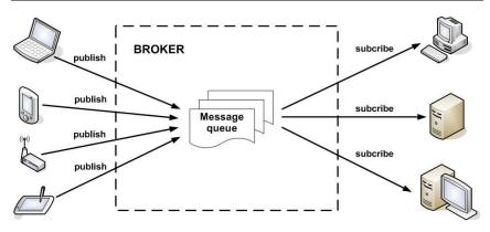
Fig. 4.5 – Architecture of MQTT
