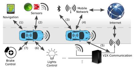
Fig. 12.7 – The information vulnerability model of the car CPS [27]:
