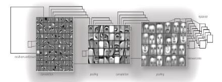
Fig. 7.21 – The general approach for face recognition by DNN
