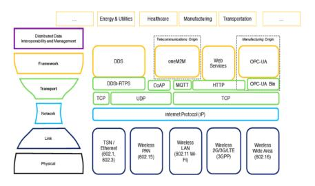
Fig. 3.7 - Industrial Internet Connectivity Stack Model
