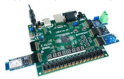
Fig. 13.5 – General view of the Nexys A7 module [17]
