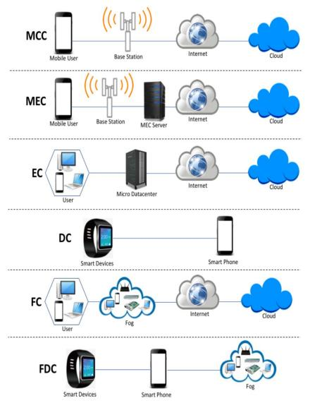
Fig. 4.11 – Architectures of MCC, MEC, EC, DC, FC and FDC.
