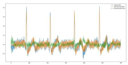
Fig. 5.8 – Original signal (blue line), reconstructed signal (yellow line) and error reconstruction (green line) using clustering
