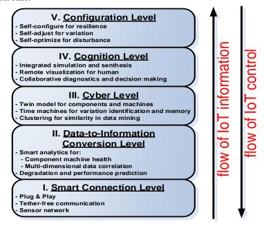
Fig. 12.1 – Five-level 5C conceptual model of CPS [20]
