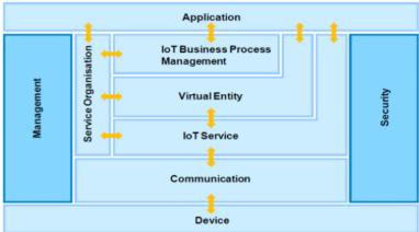
Fig. 3.2 - IoT-A Functional Model
