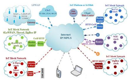
Figure 2.1. Components of IoT Architecture [25]
