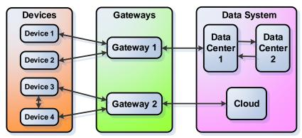
Fig. 13.6 – Three-layer D-G-S IoT architecture
