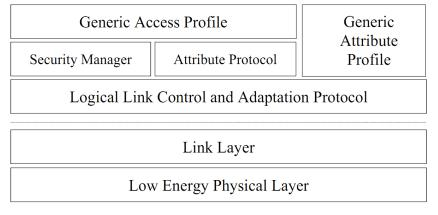
Fig. 4.4 – Bluetooth low energy single mode protocol stack
