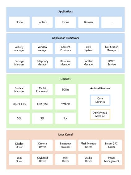
Figure 9.2 - Android system architecture
