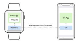
Figure 9.7 – The Watch application architecture
