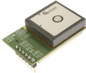
The selected module is one of the cheapest and simplest. Nevertheless, the manufacturer promises the presence of a battery for storing satellite data. An important parameter of devices connected to the Arduino – power consumption. If you overload the Arduino converter, it may burn. For the receiver used, the maximum power consumption is 45mA.
