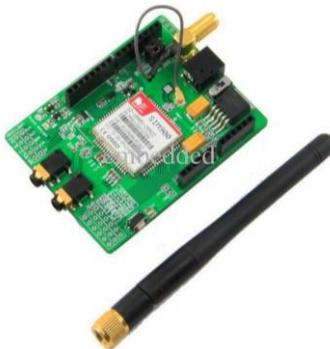
GSM module – SIM900. It supports GSM and GPRS. Neither EDGE, nor even 3G, are supported. This is probably good for transferring coordinate data – there will be no delays and problems when switching between modes, plus GPRS is almost everywhere now.
