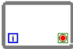
Figure 5 – While loop (LabView)
